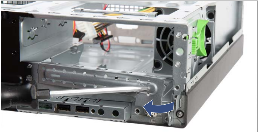
Figure 73: Removing the ODD filler cover
